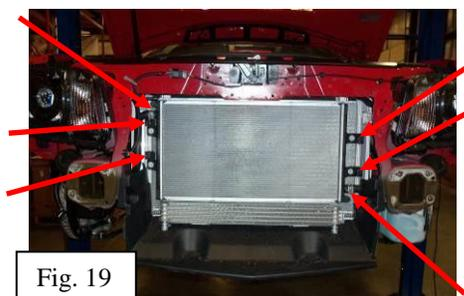
22. The heat exchanger should be removed at this time.
