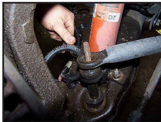
2. Disassemble / remove upper mount from vehicle (discard old bolts / nuts - new hardware is supplied in kit)
