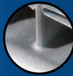
Clad Fillets on Both Sides
