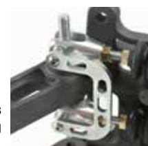
Exclusive bias "tie-bar" adds strength and sets clevis spacing for proper master cylinder function.
