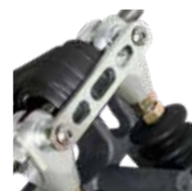
Exclusive bias "tie-bar" adds strength and sets clevis spacing for proper master cylinder function.
