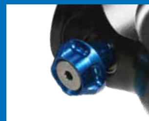
LOW SPEED REBOUND ADJUSTMENT.
